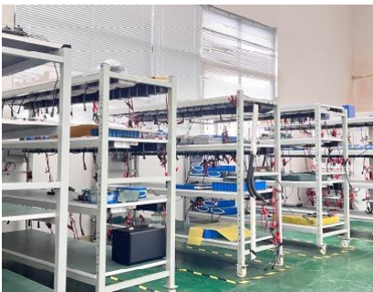
Solar street light aging line
