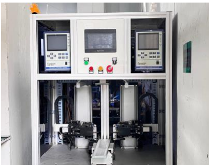
Automatic double-sided spot welder for cylindrical battery pack
